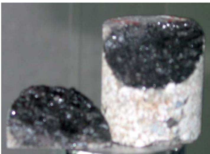
**Fig. 3 :** Sample disturbance in terms of coal intrusion in one of the tested rock specimen
