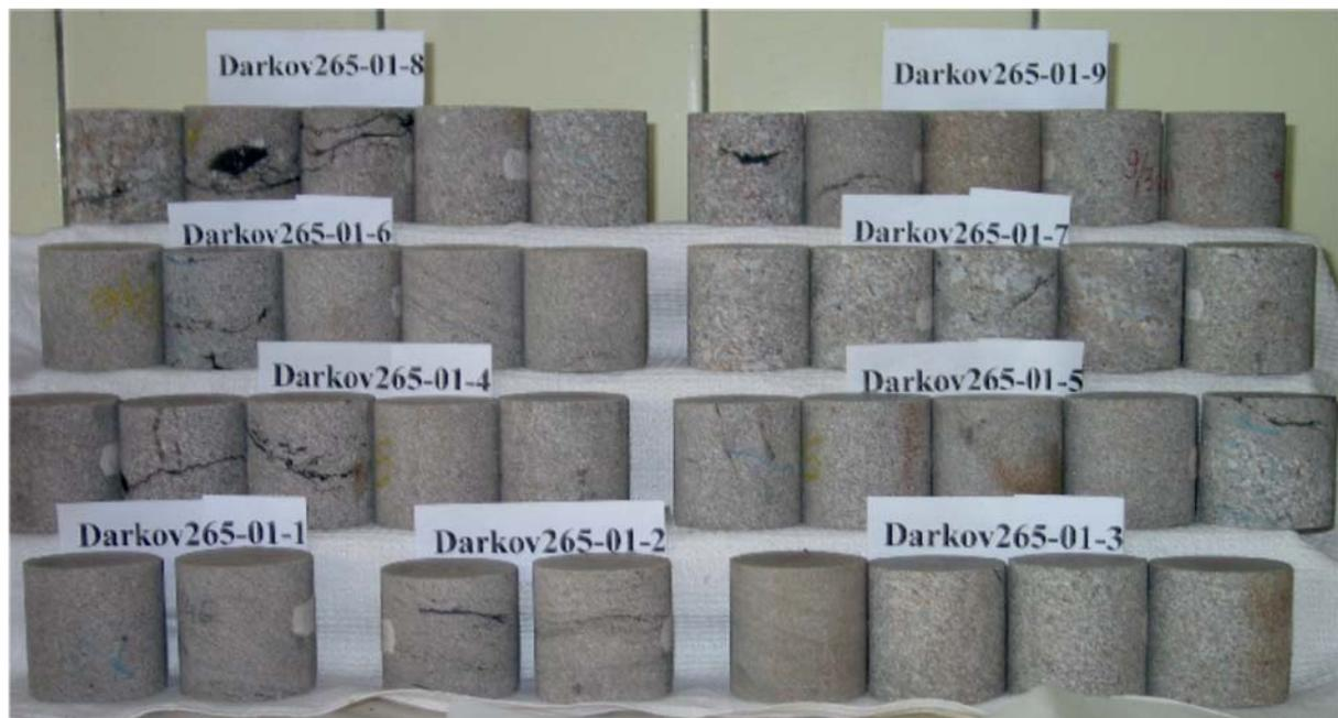
**Fig. 2** : Prepared rock specimens showing sample disturbance from borehole Darkov 265-01
