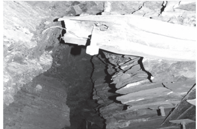
Fig. 3 : Nature of roof instability in 14 th Level at Tandsi Mine.
