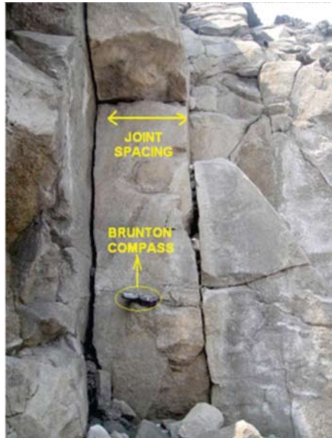
Photo 1 : Typical Joint pattern exposed within sandstone bench showing- “Joint trend”, “Joint surface”, “Joint aperture” and “Joint spacing.”
