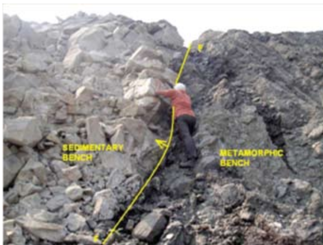
Photo 4 : A close view of major fault F1 exposed in the quarry where sedimentary benches abut against metamorphic benches
