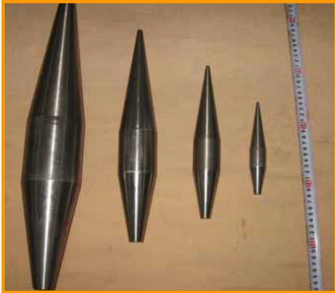
Figure 7. Strikers for dynamic size effect research
