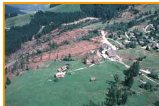
1994 Falli Hölli landslide with a displacement of 250 m in 4 months
