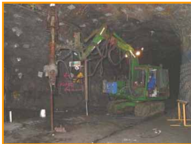
Underground over-coring rig used by Dr Rhett Hassell for his PhD research "Corrosion of Rock Reinforcement in Underground Excavations" undertaken at the WA School of Mines, Curtin University, Kalgoorlie, Australia.
