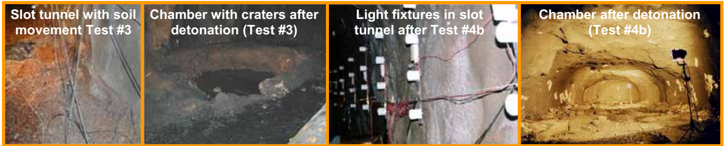
Figure 3: Photos of the detonation chamber and slot tunnel after Tests #3 and #4b
