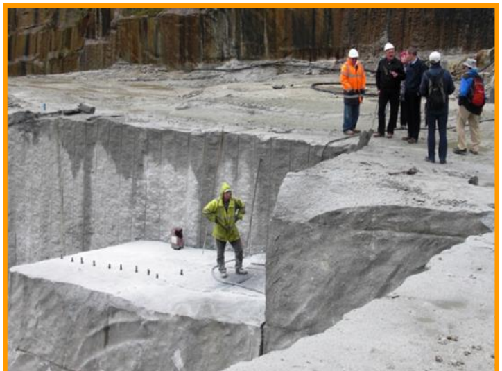
The orthogonal nature of the quarry geometry which directly reflects the orthotropic micro-structural granite anisotropy.
