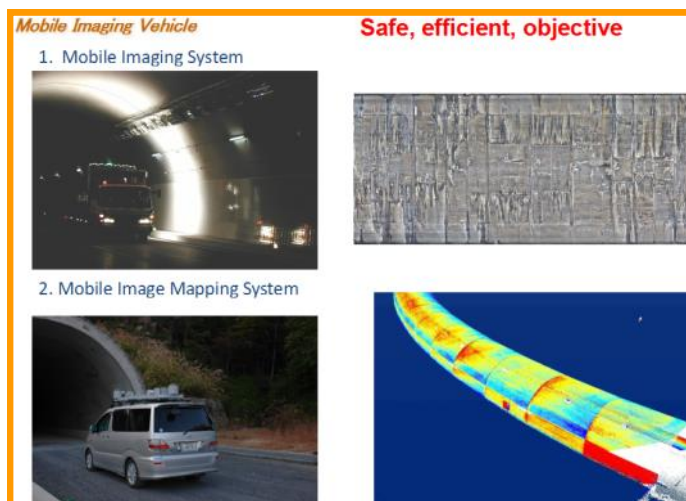
Photo 2. Mobile Imaging Vehicle for tunnel inspection and maintenance
